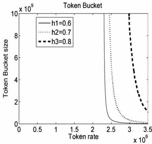
Fig. 3. Token bucket of self similar network traffic with variance  $a=561.6\text{kbps}$
