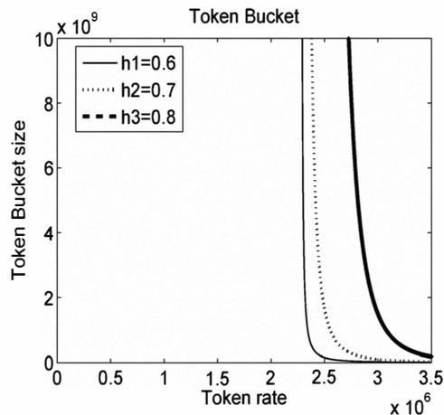
Fig. 2. Token bucket of self similar network traffic with variance  $a=280.8kbps$
