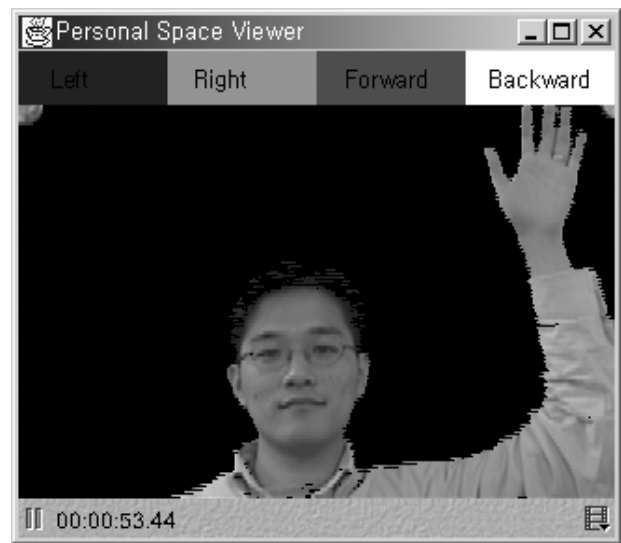
Fig.5 Personal Space Viewer : User can navigate virtual world by positioning his/her hand on each colored box at the top of the image.
