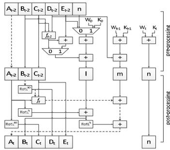
Figure 2. Base SHA-1 core architecture
